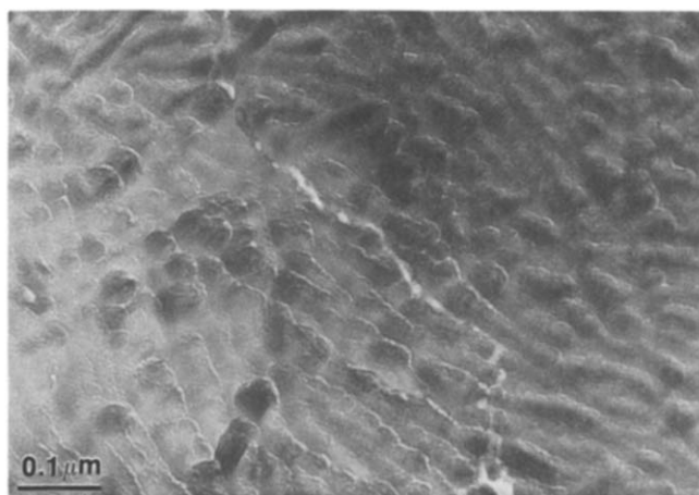
Figure 12 TEM micrograph at high magnification of portion of spherulite in spherulitic pipe showing lamellar separation
